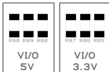
Figure 7-1 : PCI Signal Voltage Configuration Resistors (Bottom View)
