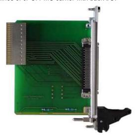
All 64 PMC I/O lines are distributed from the cPCI RJ2 connector to a 68 pin SCSI-3 type connector located in the front panel. The pin assignment corresponds to the PICMG 2.3 R1.0 PMC on CompactPCI signal mapping.
