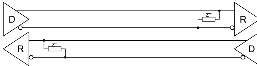
Figure 5-10 : RS422 Full Duplex Point to Point Configuration
