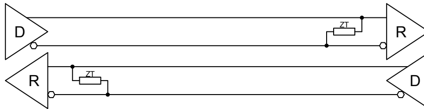
Figure 5-5 : RS422 Full Duplex Point to Point Configuration
