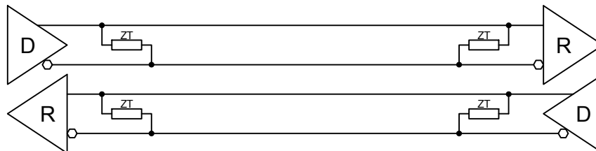
Figure 5-6 : RS485 Full Duplex Point to Point Configuration
