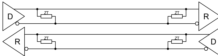
Figure 5-6: RS485 Full Duplex Point to Point Configuration
