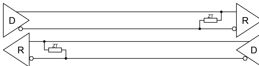
Figure 5-5 : RS422 Full Duplex Point to Point Configuration
