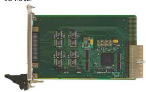
The serial communication controller is implemented in FPGA logic, along with the bus master capable PCI interface, guaranteeing long term availability and having the option to implement additional functions in the future.
