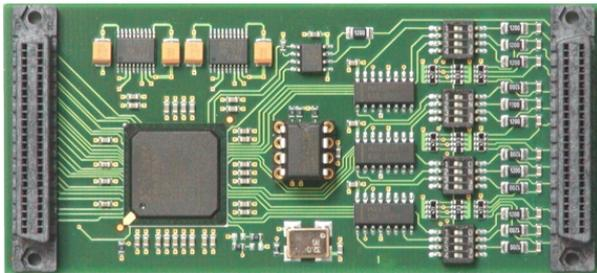
Additionally four control modes are available via the control input. The control input can be programmed to load, latch or reset the counter or it can be used as a gate for the counter clock.
