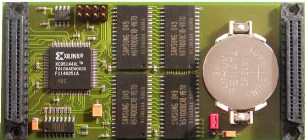
Four 512 Kbit x eight low power SRAM devices are used to provide 2 banks of 1 Mbyte (16 bit wide) SRAM memory.
