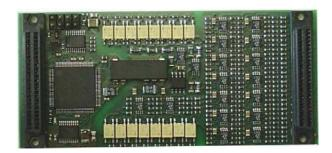
All inputs have an electronic debounce circuit. The debounce time is programmable in a range from  $900\mu s$  up to 230ms in 256 steps of  $900\mu s$ . The debounce circuit can also be disabled. The TIP606 is designed for an operating temperature from -40°C to +85°C.
