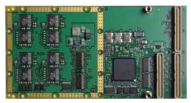
The serial communication controller is implemented in FPGA logic, along with the bus master capable PCI interface, guaranteeing long term availability and having the option to implement additional functions in the future.
