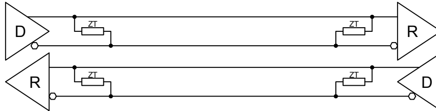
Figure 5-6 : RS485 Full Duplex Point to Point Configuration
