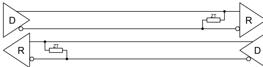
Figure 5-5 : RS422 Full Duplex Point to Point Configuration
