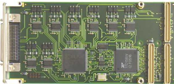
Each RS232 channel supports RxD, TxD, RTS, CTS and GND. RS422 and RS485 full duplex support a four wire interface (RX+, RX-, TX+, TX-) plus ground (GND). RS485 half duplex supports a two wire interface (DX+, DX-) plus ground (GND).
