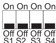
Figure 6-4 : DIP switch settings for battery backup disabled
