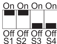
Figure 6-3 : DIP switch settings for battery backup via P14 I/O Connector
