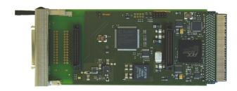
The IP power lines are fuse protected by self healing fuses and RF filtered. The operating temperature range is -40°C to +85°C.
