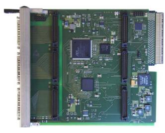
The IP power lines are fuse protected by self healing fuses and RF filtered. The operating temperature range is -40°C to +85°C.
