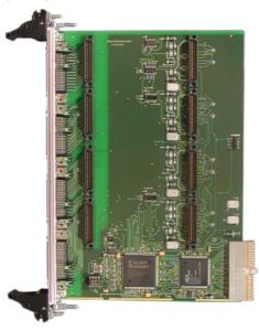
All IP interrupt request lines are mapped to PCI INTA. For fast interrupt source detection, the TCP201 provides a special IP interrupt status register.
