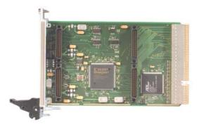
Access to all IP I/O lines is provided via J2. Status indicators for IP access, +5V and +/-12V are provided in the front panel.
