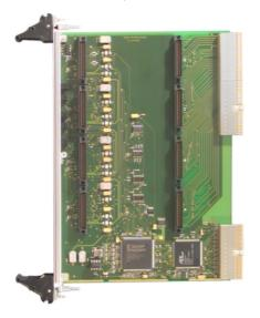
The IP power lines are fuse protected by self healing fuses and RF filtered. The operating temperature range is  $-40^{\circ}$ C to  $+85^{\circ}$ C.
