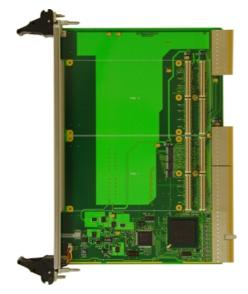
The TCP260 also provides hot swapping capability. The TCP260 on board hot swap controller controls the installation and reinstallation process of the TCP260 without powering down the CompactPCI system.
