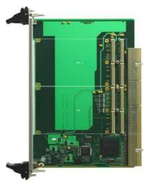
Capability of hot swapping is realized by a hot swap controller for the TCP261. The hot swap controller and the PCI-to-PCI Bridge are controlling the installation and reinstallation process of the TCP261 without power down the system.
