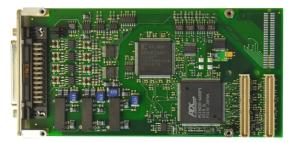
Each TPMC550 is factory calibrated. The calibration information is stored in the Identification-PROM unique to each PMC module.
