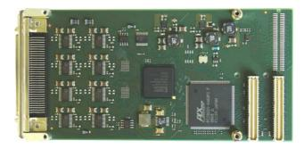
The software selectable output voltage ranges are 0-5V, 0-10V, 0-10.8V, ±5V, ±10V or ±10.8V. The output voltage range can be individually set per channel. The conversion time is typ. 10 µs and the DAC outputs are capable to drive a load of  $2k\Omega$ , with a capacitance up to 4000pF.
