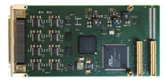
The software selectable output voltage ranges are 0V-5V, 0V-10V, 0V-10.8V,  $\pm$ 5V,  $\pm$ 10V and  $\pm$ 10.8V. The output voltage range can be set individually per channel. The conversion time is typ. 10µs and the DAC outputs are capable to drive a load of  $2k\Omega$ , with a capacitance up to 4000pF.
