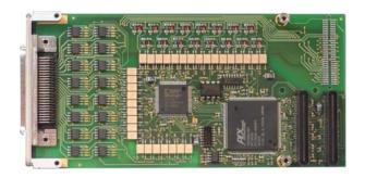
The TPMC670 has 16 / 8 digital high side switches with galvanic isolation from the computer system by optocoupler. The outputs are also isolated against each other in groups of four outputs. All outputs are protected against short-circuit and thermal overload. The output drivers are capable of driving 0.5A continuous per channel. A hardware watchdog clears all outputs in case of trigger fail. The TPMC670-1x provides front panel I/O, the TPMC670-2x provides P14 I/O.
