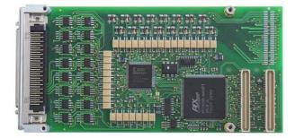
The TPMC671 has 16 digital high side or low side switches (build option) with galvanic isolation from the computer system by optocoupler. The outputs are also isolated against each other in groups of four outputs. All outputs are protected against short-circuit and thermal overload. The output drivers are capable of driving 0.5A continuous per channel. A hardware watchdog clears all outputs in case of trigger fail. The TPMC671-1x provides front panel I/O, the TPMC671-2x provides P14 I/O.
