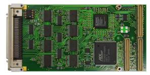
The TPMC680 supports three basic modes of operation: standard byte I/O with interrupts, 2 x 16 bit port with handshake and 1 x 32 bit port with handshake. The two handshake modes offer double buffered inputs or outputs and interlocked or pulsed handshake output protocol.
