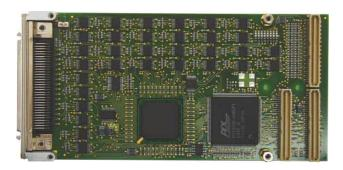
The TPMC681 provides front panel I/O via a HD68 SCSI-3 type connector and rear panel I/O via P14.
