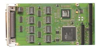
The TPMC682 provides front panel I/O via a HD68 SCSI-3 type connector and rear panel I/O via P14.
