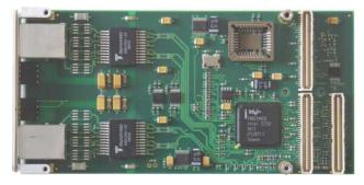
An Intel™ 82546EB Ethernet Controller (Intel™ 82546GB for ROHS compliant version) is used, which supports 10, 100 and 1000 Mbit/s transmission rates for half and full duplex operation. The TPMC884 is capable of performing an auto negotiation algorithm which allows both linkpartners to find out the best link-parameters by themselves. The TPMC884 is widely user configurable via configuration and status register access over the PCI bus. Front panel mounted LEDs indicate various network activities.
