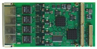
The TPMC885-10R provides four 10/100/1000Mbit/s Ethernet connections via front panel RJ45 connectors.
