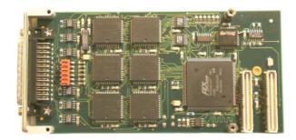
Each channel supports CAN High Speed according to ISO11898 as the physical interface. The bus line termination is selectable by a jumper separate for each bus line pair. The data transfer rates of up to 1 Mbps are supported for a bus line length of 40 m. The TPMC901-11 supports only four CAN bus channels and the TPMC901-12 has two CAN bus channels.
